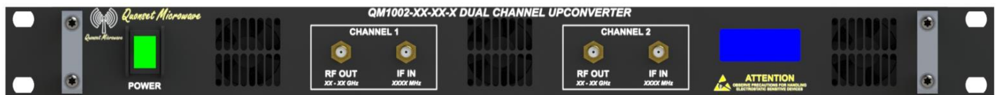
Figure 2. Front panel connections to QM1002-0.5-18.
